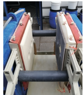
Figure 3: Separation of calcium phosphate from process water, chamber filter press with solids plate.
