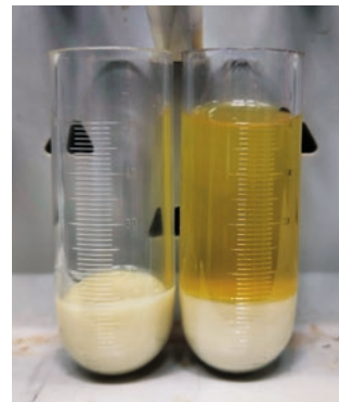
Figure 2: Separation of calcium phosphate from process water, centrifugation.
